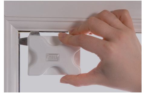
3. Position bracket behind rubber bead and carefully push the metal legs behind the bead.
