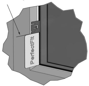
Line up the bracket with the base or top of the credit card (depending on which corner of the window you are working) and fit the bracket by pushing it between the glass and the rubber seal of the window.
