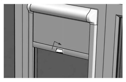
To lock the blind into position, rock the hande backwards.
