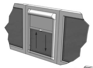
Holding the Perfect Fit handle slide the blind up and down within the frame
