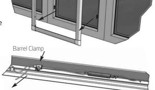
Pull the loose end of the cord through the barrel clamp to take up the slack and re-tighten the screw to hold the cord in the clamp.
