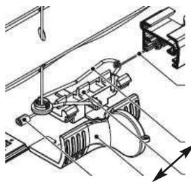
4. The operating cords are also tied off to a sliding tensioner and can be adjusted in the same way, to create the optimum tension to hold the blind in place without being too much to make it stiff to operate.
