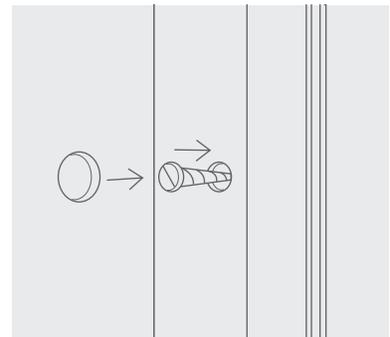
3. Insert adjustable side-guide into fixed side-guide, ensuring that the plastic bottom-bar endcap is slotted into the opening of the adjustable sideguide.
