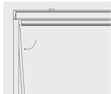
Press the adjustable side-guide into the fixed part, ensuring that the bottom bar will be free to move through it along the full drop of the blind.
