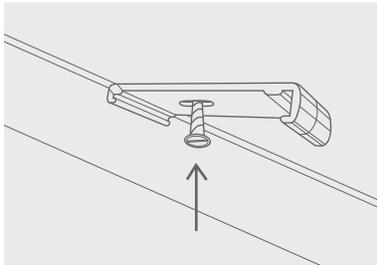
2. Set Cassette onto lip at back of bracket, as shown, and rotate into horizontal position, tight against the bracket.
