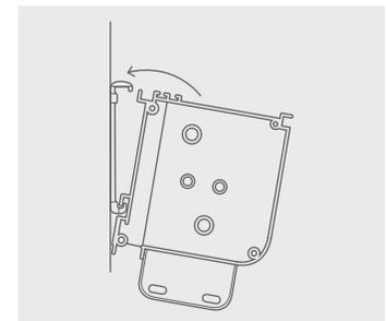
3. Slide the black plastic bracket inserts into position in each bracket, ensuring that they are fully inserted.
