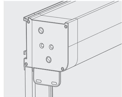
2. Once in position, screw into place at pre-drilled holes using fixings suitable for the target material.
