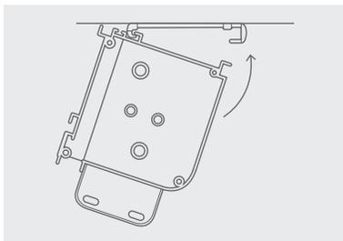
3. Slide the black plastic bracket inserts into position in each bracket, ensuring that they are fully inserted.
