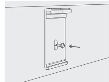
2. Set Cassette onto lower lip of bracket, as shown, and rotate into vertical position, tight against the bracket.
