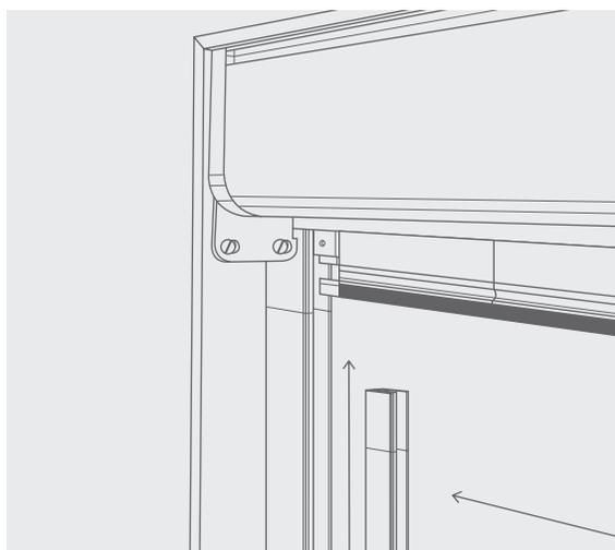
3. Press the adjustable sideguide into the fixed part, ensuring that the bottom bar will be free to move through it along the full drop of the blind.
